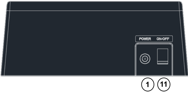
[Figure 4: Rear panel of the LTWI-BATCHG125 battery charger]
